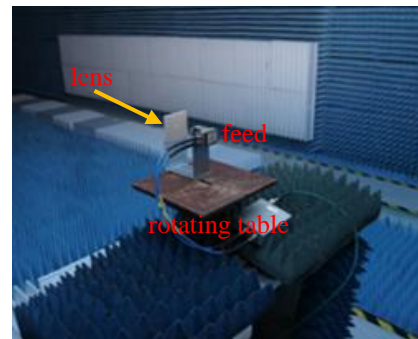
Fig. 7 Farfield radiation patterns setup.
